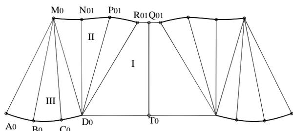
Figure 5: Unfolding of the connection which join platoval section with a symmetrical circular section
