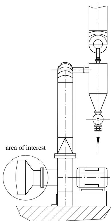
Figure 1. The schema of the dust catcher
