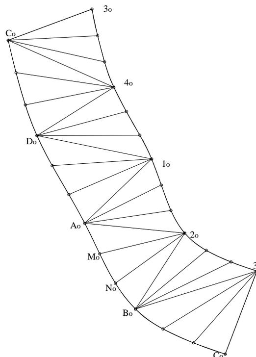
Figure 7: Unfolding of the connection which join two cylindrical sections, tangential in a point
