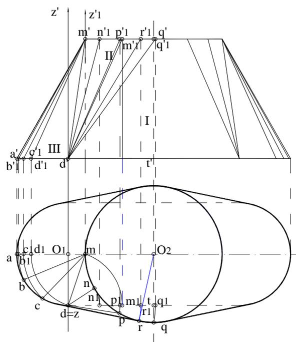
Figure 4: Double orthogonal projection of a reduction which connect a platoval section with a symmetrical circular section
