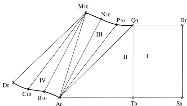
Figure 3: Unfolding of the platoval reduction with a circular section
