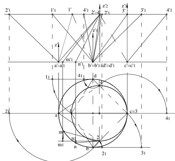
Figure 6: Double orthogonal projection of a reduction, which connect two sections of cylindrical section, tangent in a point.
