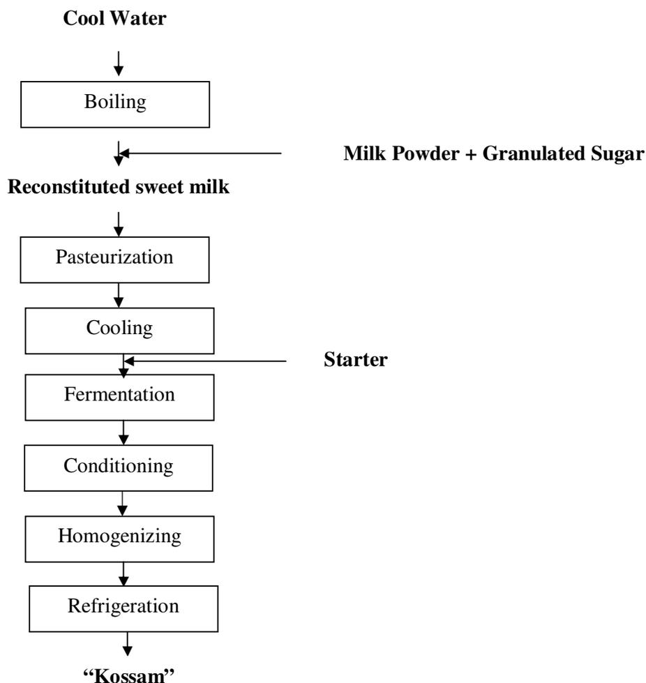
Fig. 3 Laboratory scale production of "Kossam": new flow sheet design for industrial process
