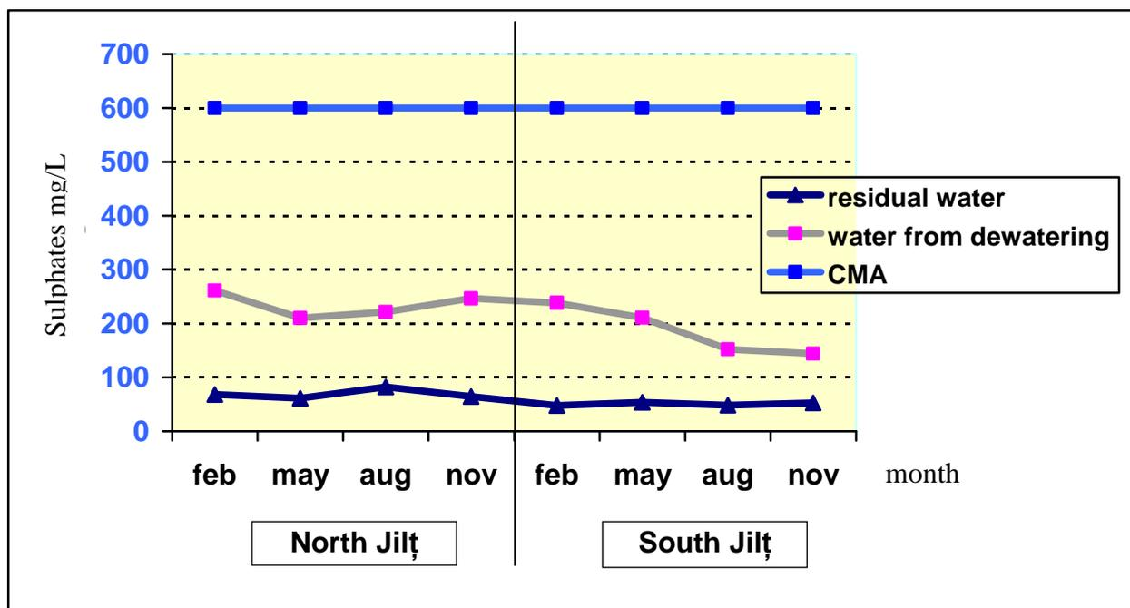
Fig.3 Variation of the sulphates in the evacuated water
