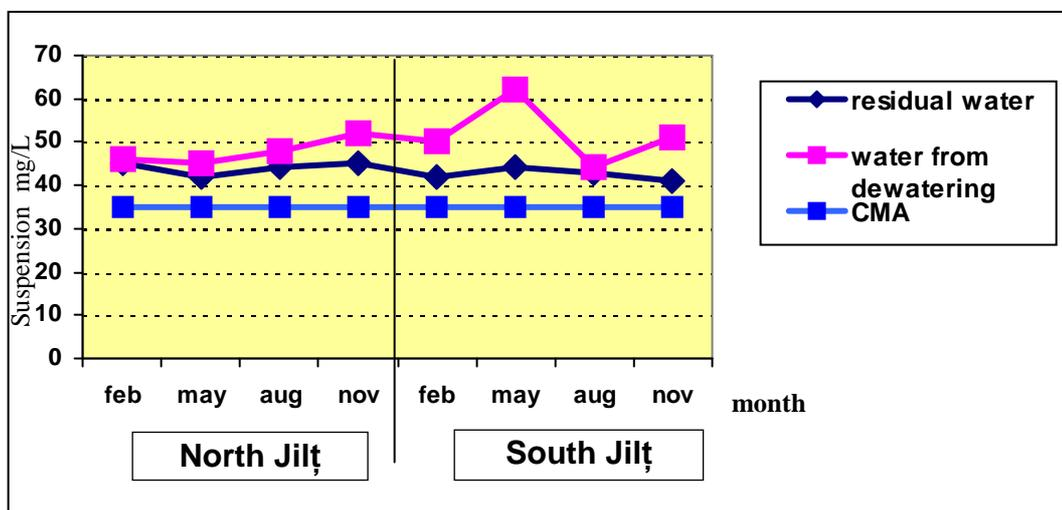
Figure 1. Variation of the total matters in suspension in the evacuated water
