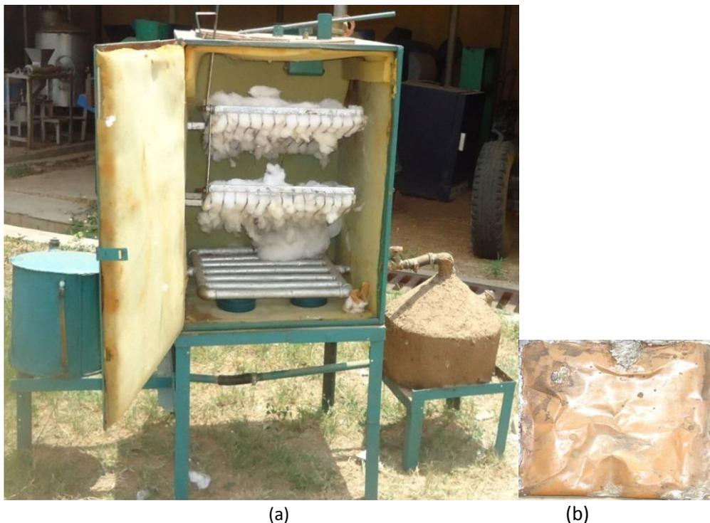
Figure 1. Illustration of (a) Experimental Rig showing the natural convective incubating system and (b) ether-capsule as temperature regulating device
