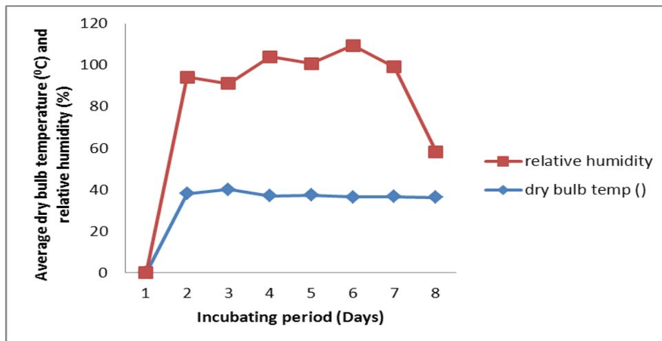
**Figure 2: Average dry bulb temperature and relative humidity against incubation period at no load**
