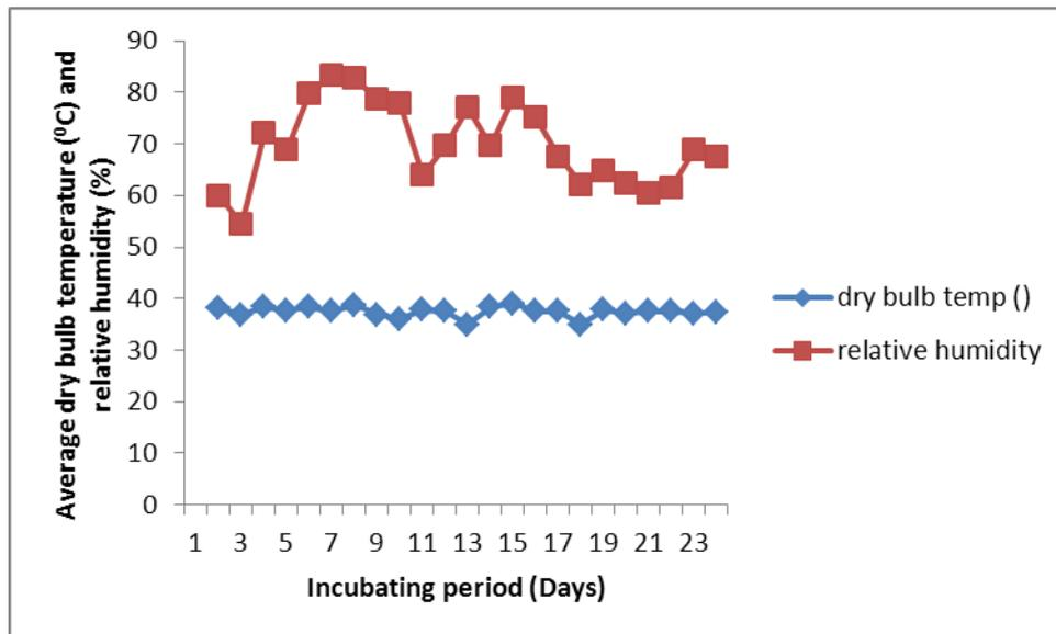
Figure 3: Average dry bulb temperature and relative humidity against incubation period when loaded (Rep I)
