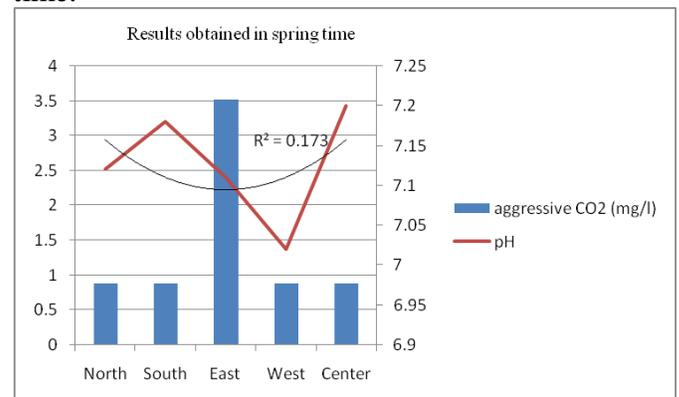
Fig. 10 The influence of pH on aggressive CO<sub>2</sub> from waters in spring time
