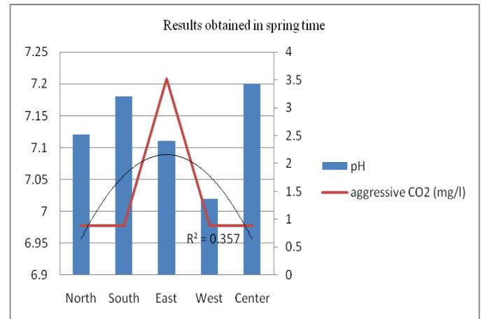
Fig. 9 The influence of aggressive CO<sub>2</sub> on pH from waters in spring time
