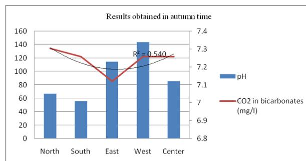
Fig. 5 The influence of CO<sub>2</sub> from bicarbonates on pH of waters in the autumn
