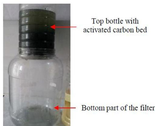
**Figure 1.** Apparatus used for active carbon filtration
