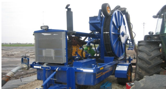
Fig. 2. Sewage-pumping plant Agrometer
