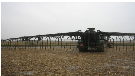
Fig. 4 Manure spreading system - Samson PG
