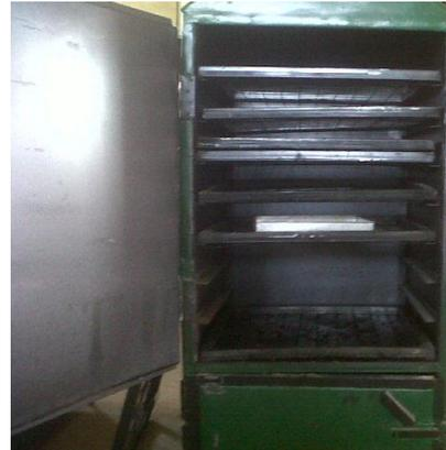
Fig. 6. Tray arrangement in Kiln
