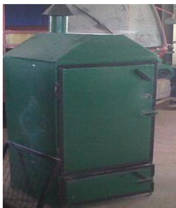
Fig. 5. NCAM fish smoking kiln
