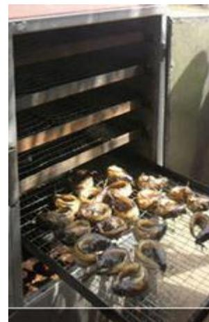
Fig. 7. Catfish inside NCAM Smoking Kiln
