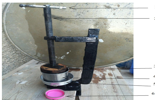
Figure 2: Manual screw press used in this work: 1- clamping bar, 2- screw, 3- wooden plunger, 4- perforated basket containing the olive paste wrapped in a cloth, 5- container- basket support, 6- oil collection vessel
